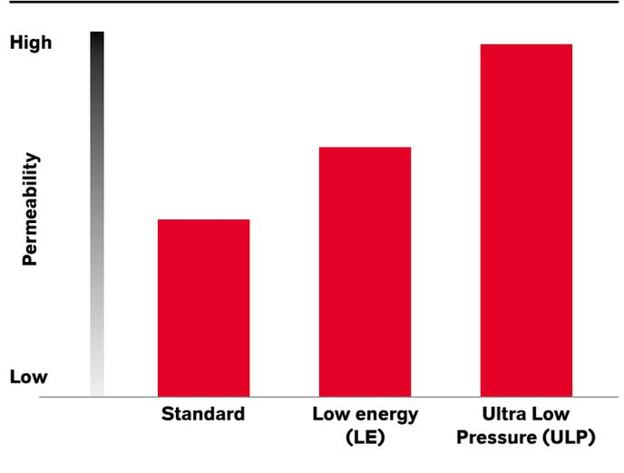
The barrier layers have a lower level of cross-linking than in LE types. ULP elements are available with diameters of 4" or 8" and with membrane surface areas of 7.9 m<sup>2</sup> or 40.9 m<sup>2</sup>. Their salt rejection under standard conditions is 99.5%.
